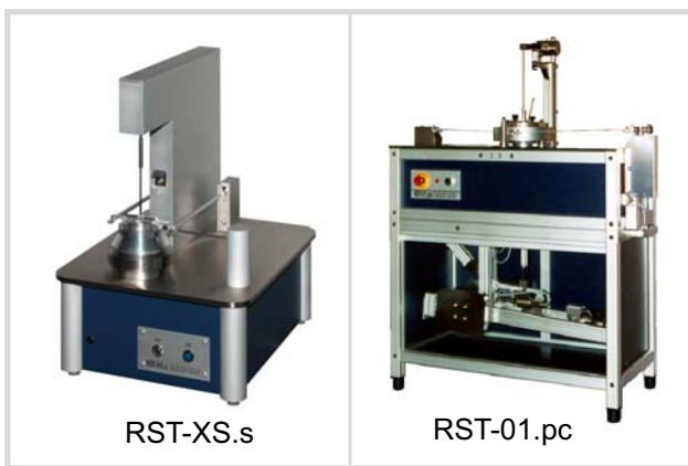
Fig. 5: Computer-controlled Ring Shear Testers RST-01.pc and RST-XS.s
